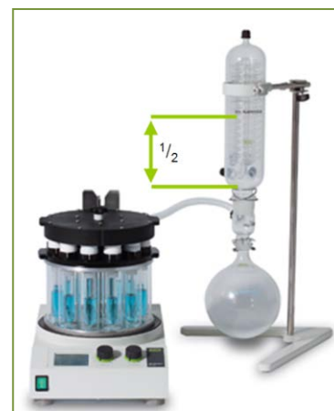
Figure 5: The vacuum and cooling conditions are ideal when the condensate covers approximately half of the height of the condenser.
