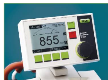
Figure 2: BUCHI vacuum controller V-855 (professional)
