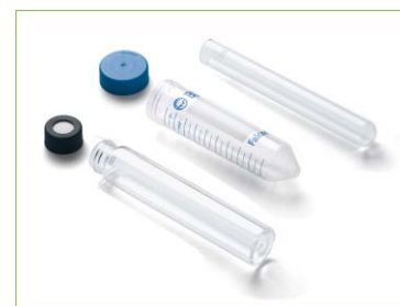
Figure 7: Selection of compatible P-12 tubes. From left: BUCHI SpeedExtractor tube, 50 ml Falcon and test tube.
