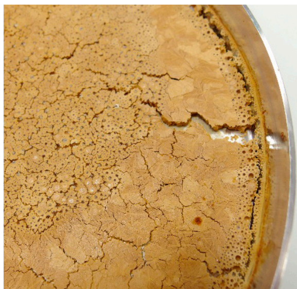
Figure 2: Dried TGY sample exhibiting a porous structure.
