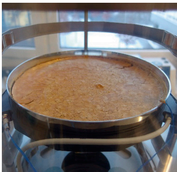
Figure 1: Steel shelf with TGY extract being dried in the Lyovapor™ L-200 Pro.
