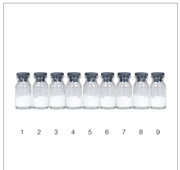
Figure 2: Freeze dried mannitol samples analyzed for its residual moisture.
