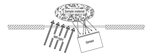
The samples should either be measured at a constant temperature or the temperature influences must be considered during calibration. Coarse grained samples should be milled before carrying out the measurement. Recommended number of scans dor a quantitative calibration: 16 - 32; granules: 64.
