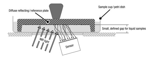
The samples should either be measured at a constant temperature or the temperature influences must be considered during calibration. Recommended number of scan for quantitative calibration: 16–32 Most liquid sample materials can be constantly analyzed with the help of a flow-cell adapter available on demand.
