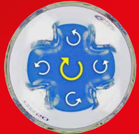
GS vessel principle (viewed from above)
