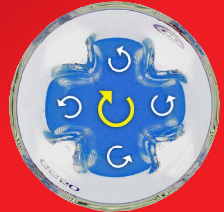
GS vessel principle (viewed from above)
