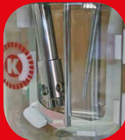
Dispersing aggregates, PTFE anchor stirrer and temperature probe
