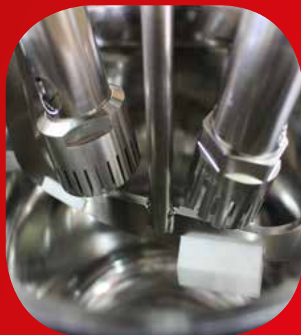
Design with two special dispersing aggregates
