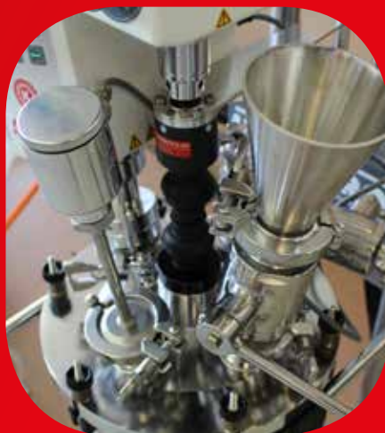
tri clamp connectors and dosage funnel on the lid
