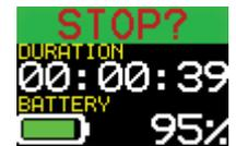
Colour coded display showing remaining battery life
