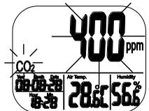
The calibration will require approximately five (5) minutes. When the calibration is complete, the blinking stops and the meter returns to the normal operating mode. Press ESC to abort a calibration session (not recommended).
