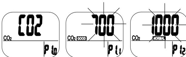
Press the ▲ or ▼ button to increase or decrease the value. Each press adjusts in 100 ppm increments. The range is 0 to 700 ppm (default is 700 ppm).
