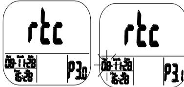
Press the ▲ button from P3.2 to access P3.3. The current DATE (day) setting will blink. To change the day, press the ▲ or ▼ button. Press the SET button to save the setting and move to P3.4 (or press the ESC button to return to P3.0 without saving).
