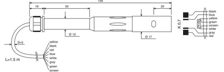
**SPTKI10:** Industrial conductivity probe in glass with 2 platinum electrodes, S7 - PG13.5 connector, **cell constant K = 1**, temperature working range 0...100 °C.
