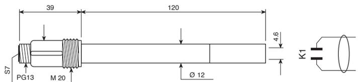
**SPTKI11:** Combined industrial conductivity and temperature probe in Rytron with 2 platinum electrodes, 3/4" BSP connector, 5 m cable, **cell constant K = 1**, 2-wire Pt100, temperature working range 0...80 °C.
