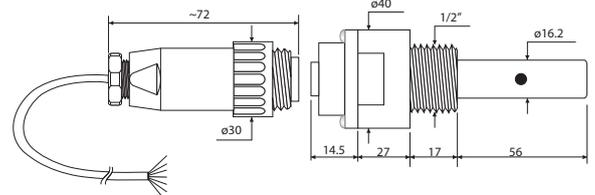
**SPT86:** 4-electrode combined conductivity and temperature probe with Pt100 sensor. **Cell constant K= 0.7**, 1.5 m cable, temperature working range 0...90°C.
