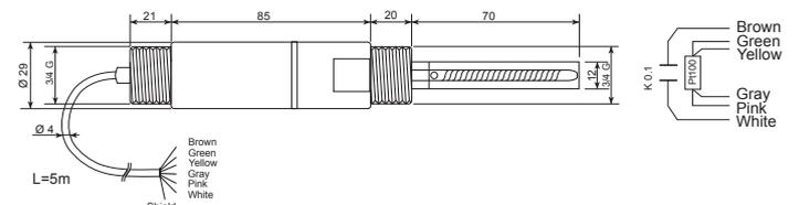
**SPTKI13:** Combined industrial conductivity and temperature probe in Rytron with 2 platinum electrodes, 3/4" BSP connector, 5 m cable, **cell constant K = 10**, 4-wire Pt100, temperature working range 0...80 °C.
