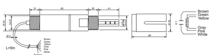
**SPTKI12:** Combined industrial conductivity and temperature probe in Rytron with 2 platinum electrodes, 3/4" BSP connector, 5 m cable, **cell constant K = 0.1**, 4-wire Pt100, temperature working range 0...80 °C.
