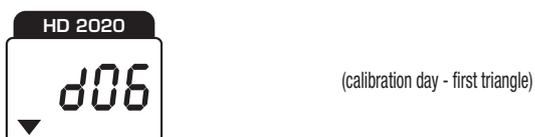
With the SETUP button switch setting the date of calibration with the lighting of the second triangle to the left and display the number of years of calibration. You can type the number of years and months between the date of calibration, entered by the laboratory conducting the formal point and the expiry date.
