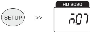
Use the arrows to increase / decrease the value. With the SETUP button is confirmed and passed to the current day:
