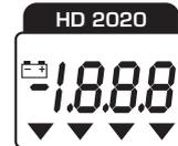
...an auto-test including the level of battery charge starts and brings the instrument to the standard working condition.
