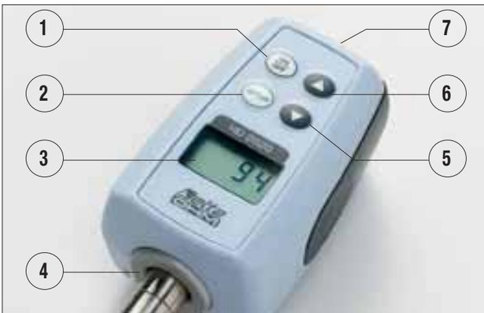
The clock/calendar allows you to set the number of years and months of validity of the calibration from the date of adjusting: at the expiration time, an appropriate symbol flashes on the display.
