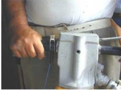
These pictures show the possibility to mount the sensor for two different handles categories. The ISO standard 5349-1 specifies the orientation of the reference system according to which are to be collected the three acceleration's vector
