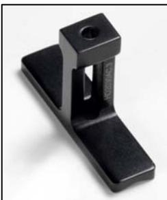
The HD2030AC4 is an adapter to be held between the hand and the handle. The accelerometer is placed in central position between the middle finger and the ring finger or between the index and the middle fingers. Light alloy made, it is suitable for anatomical shape, non-cylindrical and/or small dimension handles.
