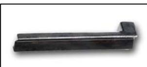
The HD2030AC2 is made of light alloy and fitted with accelerometers using a threaded hole (10-32 UNF or UNC 5-40); accelerometer is secured by a screw on the adapter.
