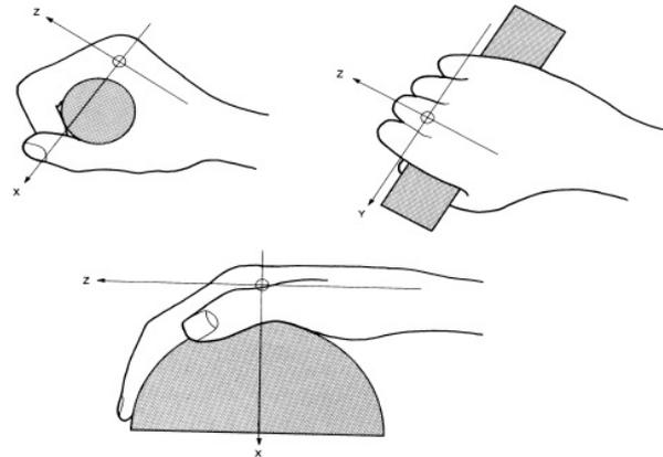
Since the ISO 5349-1 introduced as evaluation parameter the accelerations vector sum, the orientation of the coordinate system, purely conventional, does not affect the evaluation procedure; it is therefore independent of the reference system adopted.
