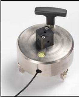
Support suitable for vibration measurements on floors and other surfaces.
