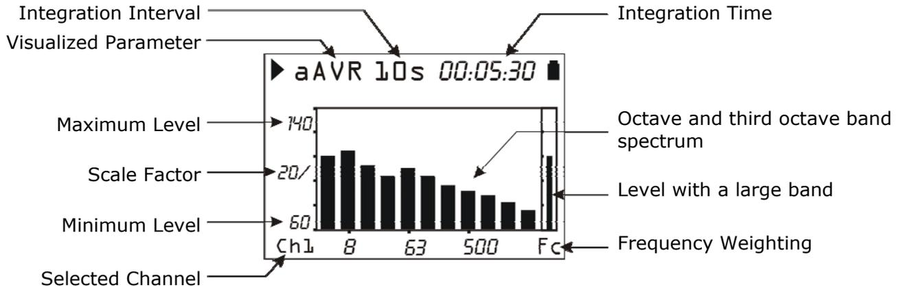
The SPECTRUM screen presents in graphic form the octave or third-octave bands spectrum related to each of the 3 measurement channels. The order of the visualized spectrum, in octave or third-octave bands, is set entering the Menu >> Parameters >> Spectrum Analyzer >> Order.
