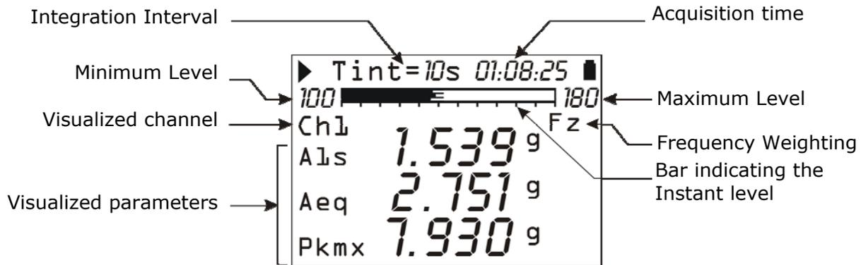
The VLM screens shows, in numerical form, three frequency weighted parameters related to each of the three measurement channels or to the acceleration vector calculated with the data of the first three axes. **It is possible to scroll in sequence the screens using the right and left cursor keys.**
