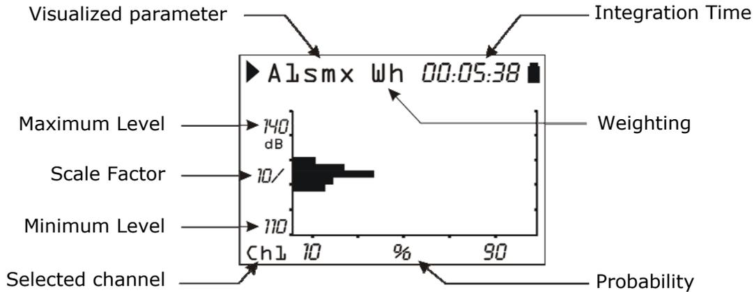
The PROBABILITY screen presents in graphic form the probability distribution of the values of the parameter visualized in the PROFILE screen for each of the 3 channels.
