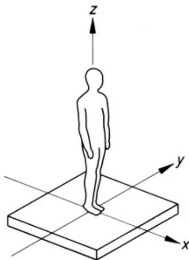
The recorded magnitude is the r.m.s. weighted acceleration value (Root mean square value) in the frequency range from 0.5 Hz to 80 Hz. Below 0.5Hz the body, as a single mass, homogeneously follows the displacement of the vibrating surface with which it is in contact to. Higher frequencies than 80Hz involve only the surface of the body where the contact is; deeper layers of the epidermis leads to a rapid attenuation of vibrations not reaching internal structures of human body.
