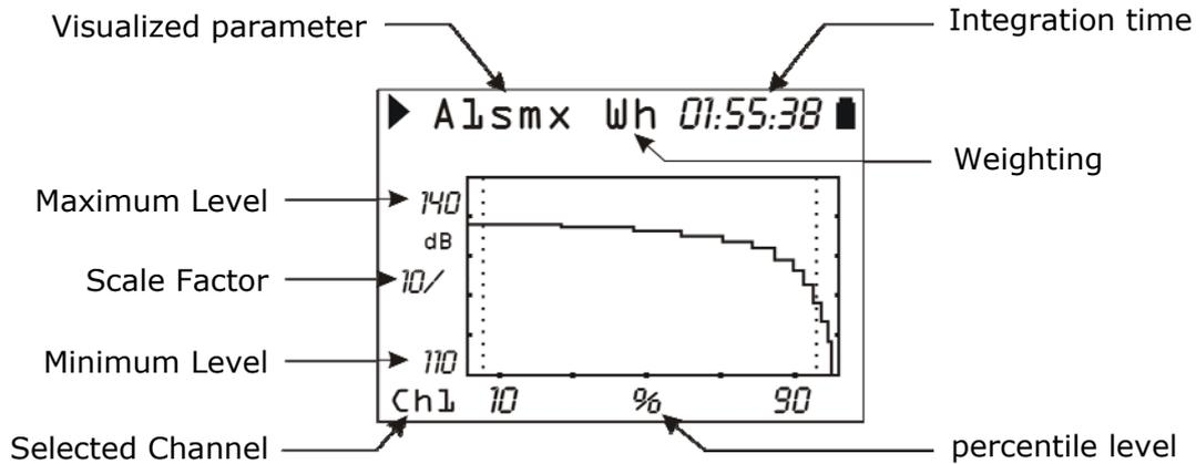
Percentile screen presents in graphic form the percentile levels from  $L_1$  to  $L_{99}$  associated with the parameter visualized in the PROFILE screen for each of the 3 channels.
