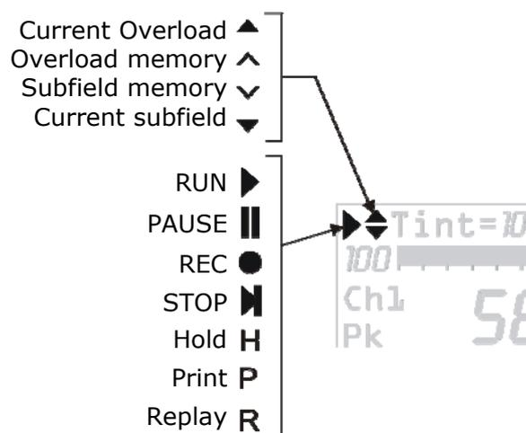
The first symbol in the top left corner of the display indicates the **acquisition status** of the vibration analyzer.
