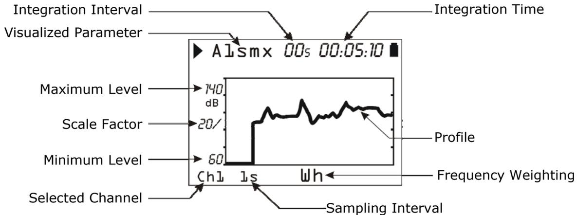
This screen presents in graphic form the profile of a frequency weighted parameter related to each of the 3 measurement channels.
