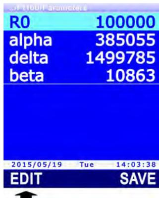
**Fig. 13.1.3: parameters for temperature calculation equation**
