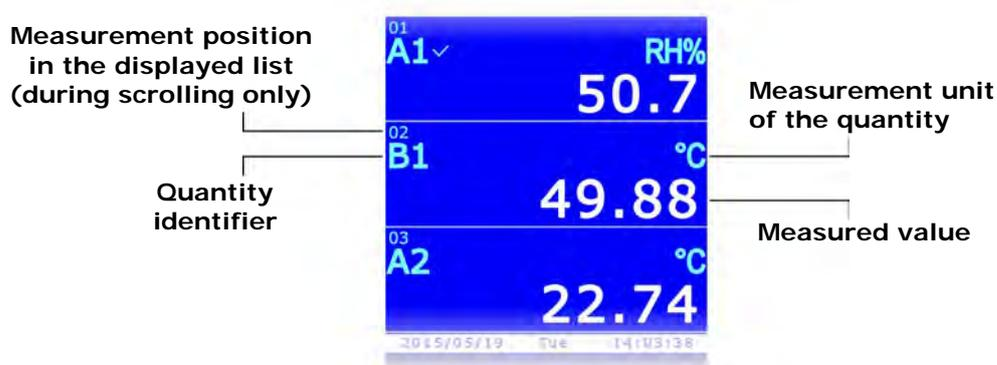
Fig. 3.2: measurements display
