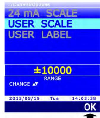
3. Set the minimum value of the voltage or current signal (e.g. 4 mA, point X1 of the example at Fig. 13.6.1). Set the first digit using ▲ and ▼, then select the "-->" command (**F2** key) to move to the next digits (the currently selected digit flashes). To return to a previous digit, select the "<--" command (**F1** key). After setting all the digits, press **OK** (**F3** key) to confirm the value.
