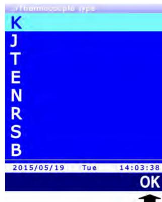
**Fig. 13.2.1: selecting the type of thermocouple**
