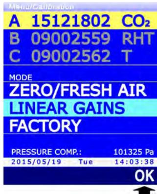
Fig. 13.5.1: calibrations for CO<sub>2</sub> probes
