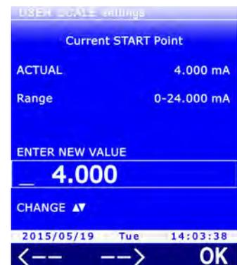
4. Set the maximum value of the voltage or current signal (e.g. 16 mA, point X2 of the example at Fig. 13.6.1). Set the first digit using ▲ and ▼, then select the "-->" command (**F2** key) to move to the next digits (the currently selected digit flashes). To return to a previous digit, select the "<--" command (**F1** key). After setting all the digits, press **OK** (**F3** key) to confirm the value.
