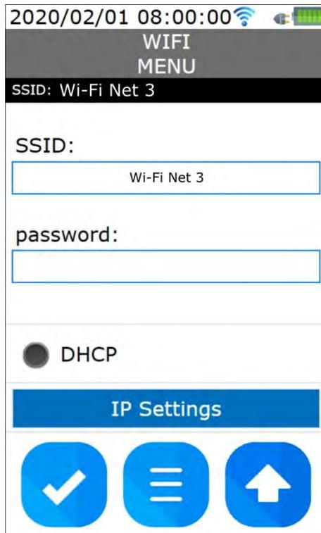
Select DHCP (Dynamic Host Configuration Protocol) to automatically get a dynamic IP address from the network. After connection, the dynamic address assigned by the network to the instrument is visible by pressing "IP Settings". To enter a static IP address manually, deselect DHCP and press "IP Settings", then configure the address and confirm by pressing the "check" key.
