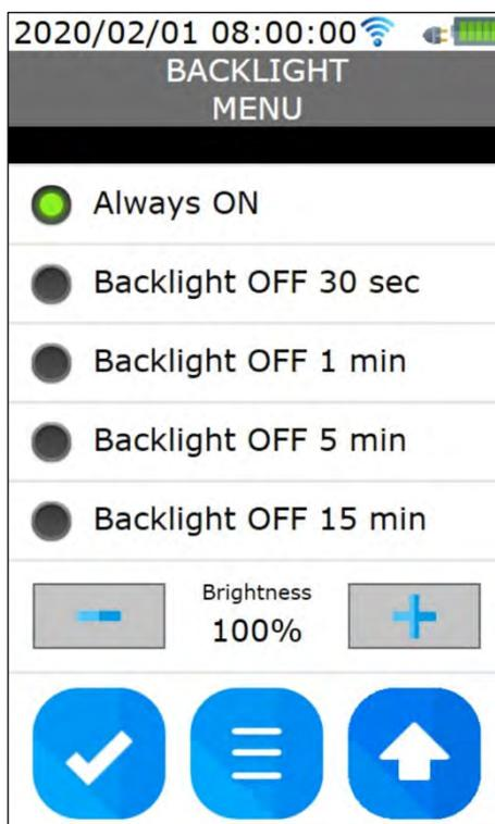
Use the +/- keys to adjust the display brightness. The lower the display brightness, the longer the battery autonomy will be.
