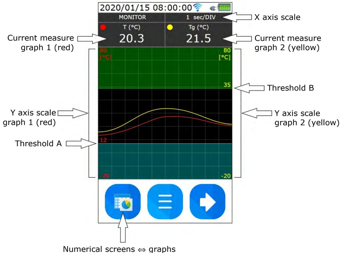
The thresholds are represented by a blue line (threshold A) and a green line (threshold B). The value of a threshold is shown on the Y axis of the quantity to which the threshold is associated. The area of the graph that exceeds the threshold values can optionally be highlighted with a shadow.
