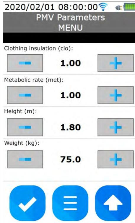
Set the clothing insulation (in CLO), the metabolic rate (in MET), the height and weight of the individual by using the +/- keys.
