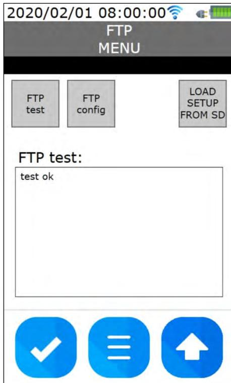
The configuration of the FTP connection can be entered using the virtual keyboard of the instrument or it is possible to load the configuration from a text file present in the instrument memory. In order to configure the FTP connection, select "FTP Config", then fill in the fields: FTP address, port number, user name, password (by pressing on the word "Password", the password can be made clearly visible or hidden) and data destination folder. Press the "check" key to confirm.
