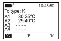
The battery charge symbol and current time are up on the left (for further details, see page 32).
