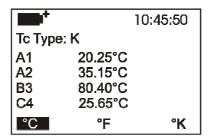
If a probe is disconnected when the instrument is on, the value on the display is replaced by a series of dashes: Reconnect the probe to view the new data.
