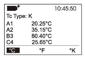
The first area displays, from top to bottom, the **battery's charge status** and the current **time**, the **type** of selected thermocouple, and the **temperatures measured** by the probes connected to the inputs.
