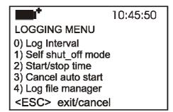
You can set the data capture frequency (*Log interval*) and the automatic logging start (*Start/stop time*). The capture interval is the same for all probes. With the "Log File Manager" you can handle the stored data sessions: printing, erasure.
