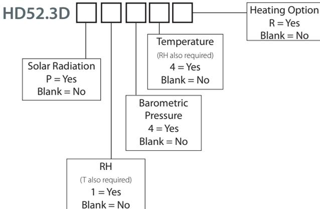
**HD52.3D...** 2-axis ultrasonic static anemometer for the measurement of wind speed and direction, U-V Cartesian components of wind speed, Wind Gust, relative humidity and temperature (optional), global solar radiation (optional), barometric pressure (optional) and rainfall (optional). **The "rainfall" and "global solar radiation" options are alternatives.** Equipped with compass.
