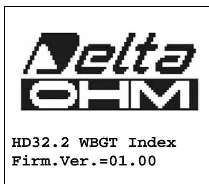
In addition to Delta Ohm logo are indicated the instrument code and the firmware version.
