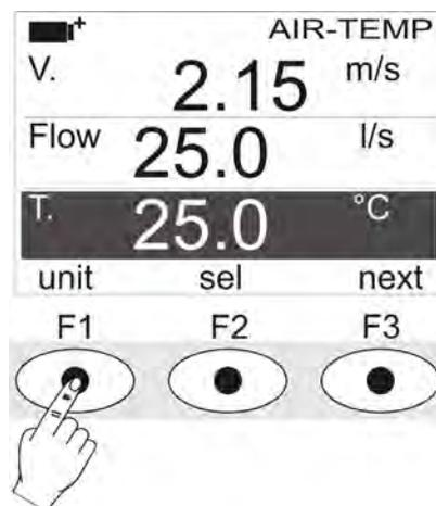
By pressing **F3** with **next** on the last line, you go to the **light probes** complete with SICRAM module:
