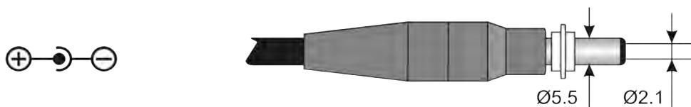
The external diameter of power supply connector is 5.5 mm, the internal diameter is 2.1 mm.
