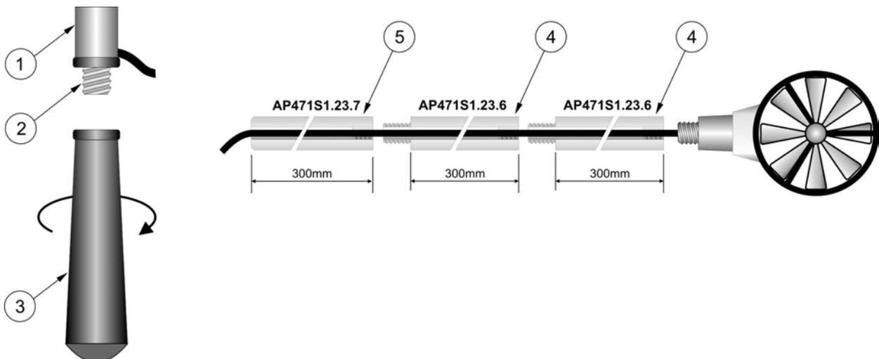
The **AP472S1 - AP472S2** probes, in addition to the telescopic rod with swivel head can use the rigid telescopic rod  $\varnothing 16$  mm. Unscrew the handle (3) holding the probe body still in the point (1). Screw the rod end **AP471S1.23.6** (4) on the screw (2). You can add more telescopic rods **AP471S1.23.6**. The last element can be the handle (3) or the telescopic rod **AP471S1.23.7** (5).
