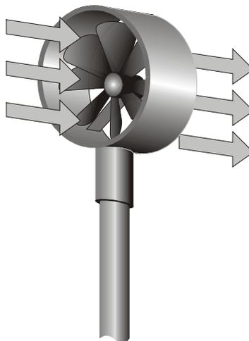
The probe should be maintained orthogonal to the flow and not tilted in relation to it:
