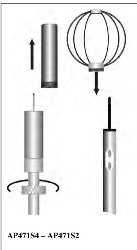
The AP471S1 and S3 probes are fitted with a cylindrical protection screen that can slide longitudinally over a groove. The screen has two end-of-travel positions that block it in measurement condition (completely low) or rest condition (completely high). To reduce the space occupied when not used, the AP471S2 and AP471S4 are supplied with a protection cylinder that can be screwed on the probe's head.
