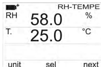
The first display line shows “**RH-TEMPE**” indicating that the measurements of a **combined humidity/temperature probe** complete with SICRAM module are displayed.
