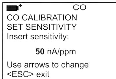
9. With Up and Down arrows set the sensor sensibility value. Press ENTER to confirm: the instrument comes back to the previous screen.
