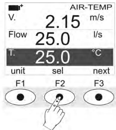
By pressing **F1** when the second line is selected, you can change the wind speed unit of measurement:
