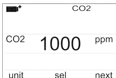
The first line of the display indicates the acronym “**CO2**”, indicating that the measurement of **carbon dioxide concentration** detected by the **CO2 probe** with SICRAM module is visualized on the display.
