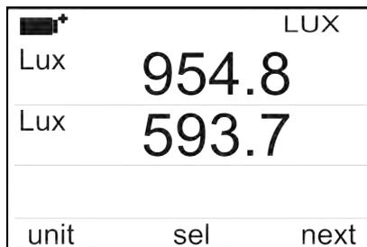
The first display line shows “**LUX**” indicating that the measurement of a **light probes** complete with SICRAM module are displayed.
