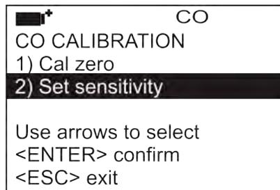
8. With Up and Down arrows select “Set sensitivity” and confirm with ENTER. The screen for the replacement of CO sensor appears.
