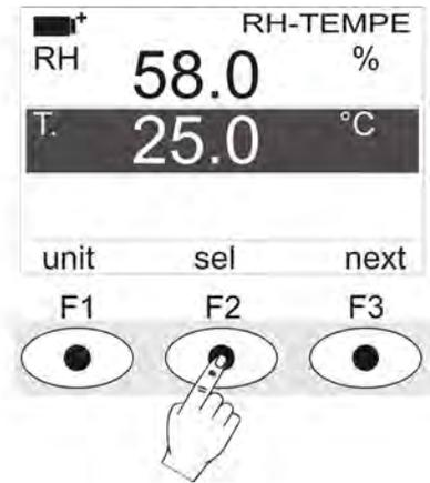
By pressing **F1** when the second line is selected, you can change the relative humidity unit of measurement:
