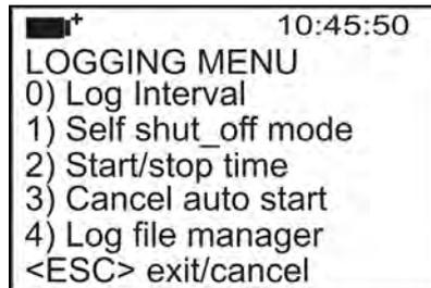
You can set the data capture frequency (*Log interval*) and the automatic logging start (*Start/stop time*). **The capture interval is the same for all probes.**
