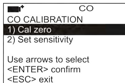
4. With Up and Down arrows, select "Cal zero" and confirm with ENTER. The screen for the calibration of CO sensor appears.
