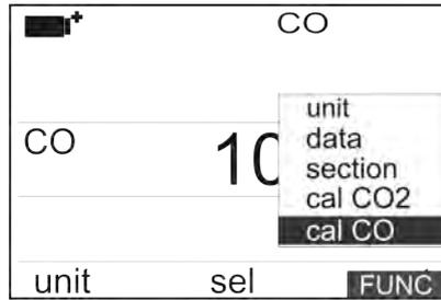
7. The screen for the operation to done on the sensor appears (calibration or replacement):
