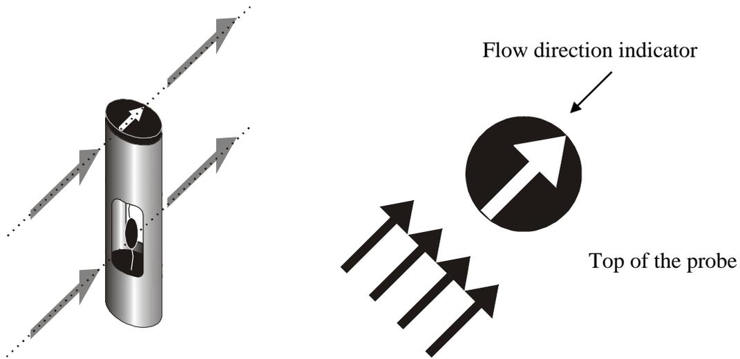
The probe should be maintained orthogonal to the flow and not tilted in relation to it:
