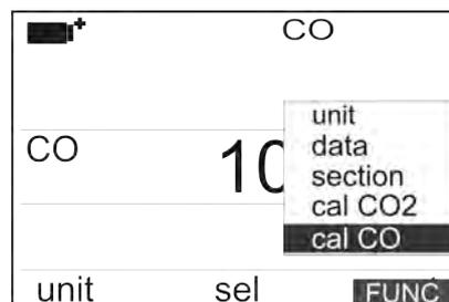
4. The screen for the operation to execute on the sensor appear (calibration or replacement):
