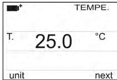
The first display line shows “**TEMPE.**” indicating that the temperature of a **Pt100 probe** complete with SICRAM module is displayed.
