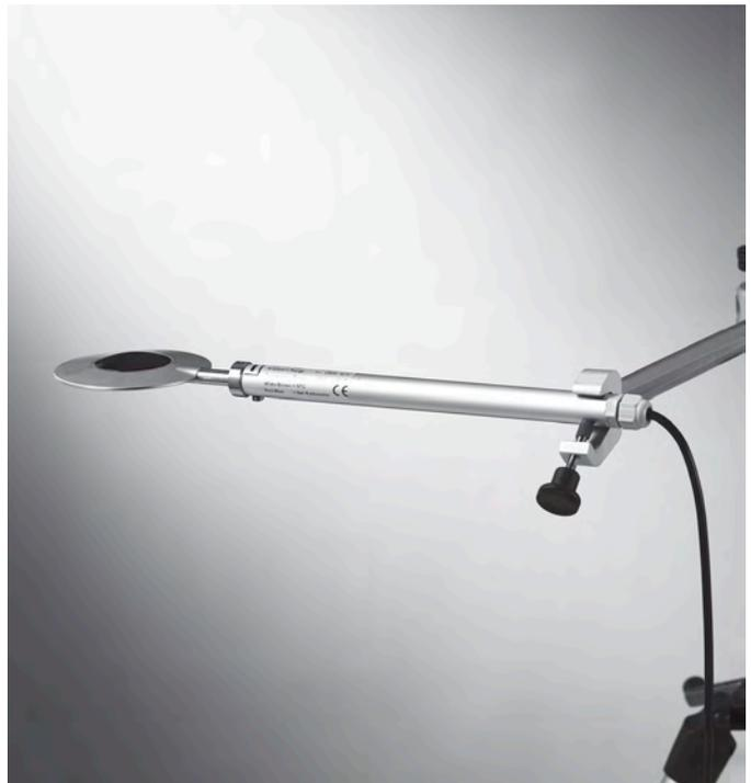
The face of the probe marked by the symbol
