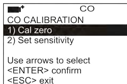
5. With Up and Down arrows select “Cal zero” and confirm with ENTER. The screen for CO sensor calibration appears.
