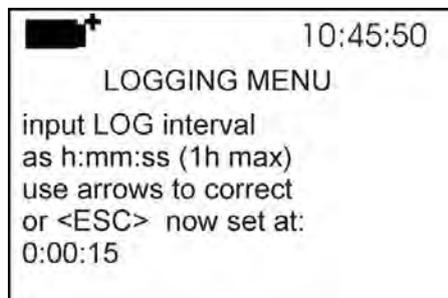
1. Use the arrow keys **▲ ▼** to select the interval duration from 15 seconds to one hour;
