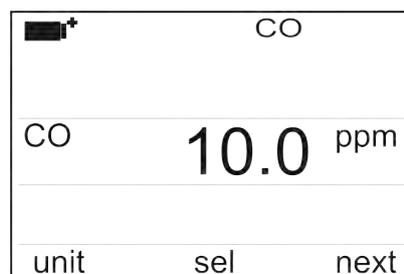
The first line of the display indicates the symbol “**CO**”, indicating that the measurement of **carbon monoxide concentration** detected by the **CO probe** with SICRAM module is visualized on the display.
