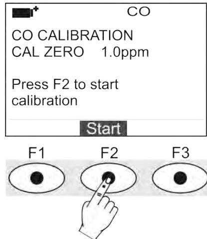
Next to “CAL ZERO” writing is indicated the CO concentration value measured by the instrument.
