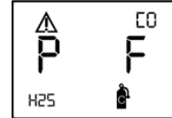
Calibration results (H2S pass; CO fail)
