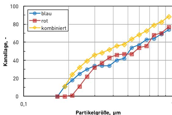
Assignment of channel position to particle size depending on the wavelength used (blue 450 nm, red 660 nm, combined).
