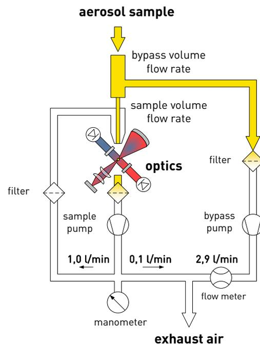
Schematic description of the operating principle of the LAP 323.
