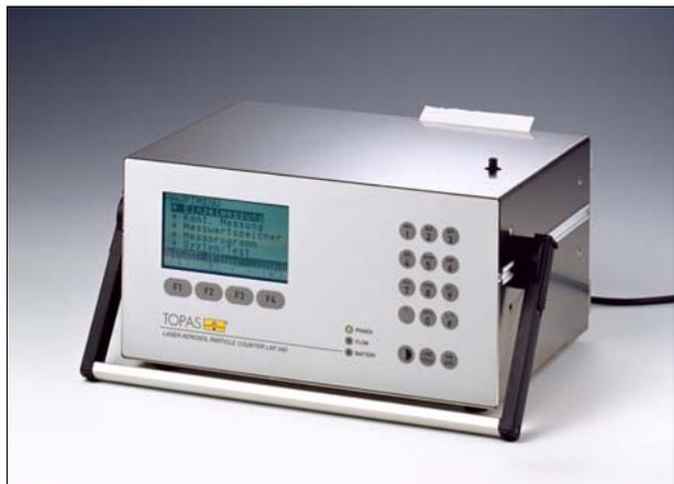
Laser Aerosol Particle Counter LAP 340
